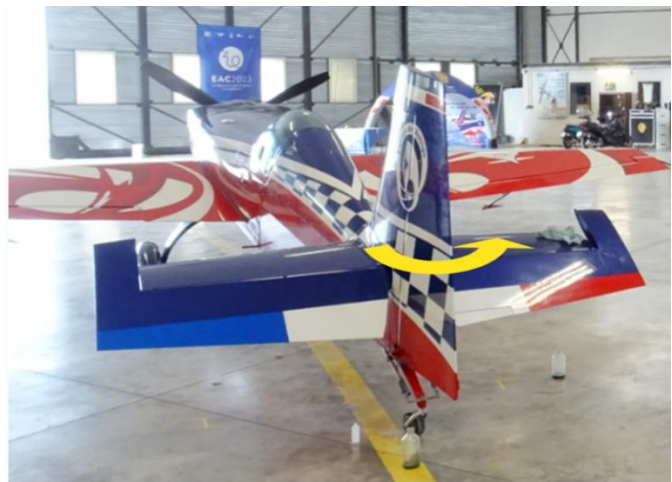
Figure 12 : illustration of the "left-right" bending effort on the rudder.
